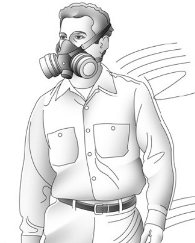
Half mask Elastomeric Respirator APF=10 Needs to be fit tested
