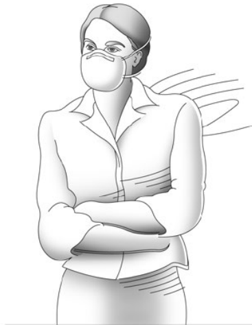
Half mask Filtering Facepiece Dust mask APF=10 Needs to be fit tested
